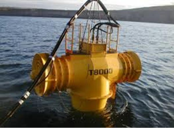
Figure 5.7 Mass flow excavator (James Fisher Marine)
