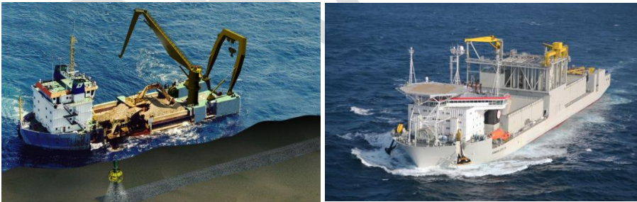
Figure 5.18 Typical Rock Placement Vessel
