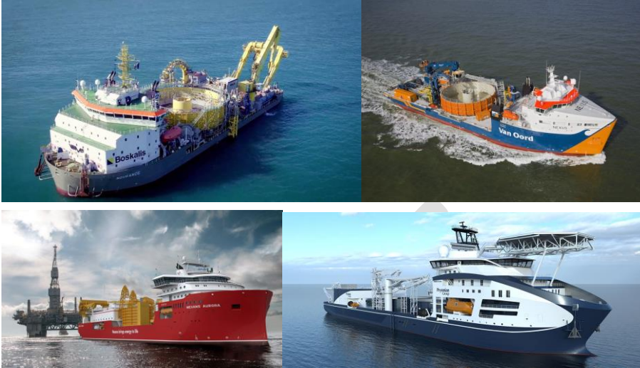
Figure 5.17 Typical Cable lay Vessels
